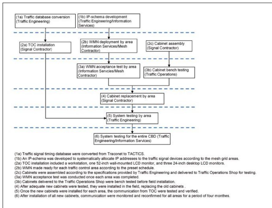
Figure 3. Work plan of CBD signal system upgrade.
